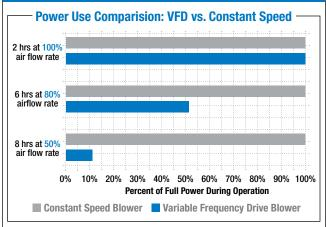
Conventional fan drives run at a constant speed even if the required static pressure at the collection area is higher or lower than that provided by the fan. This imbalance between power needed, and power provided, is the cause of wasted energy in constant-speed fans.
